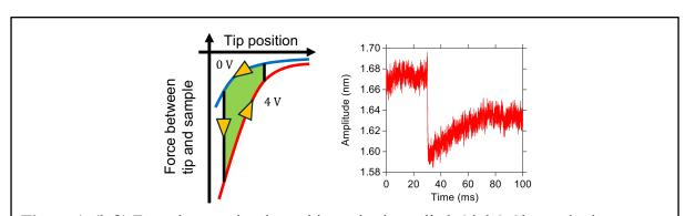
**Figure 1.** (left) Force hysteresis when a bias pulse is applied. (right) Change in the oscillation amplitude showing the cantilever's energy loss associated with a bias pulse.
